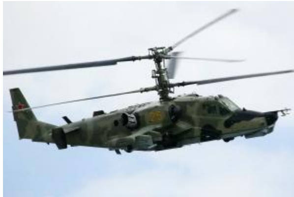
KAMOV Ka-50 "Black Shark" with distinctive coaxial rotor system
