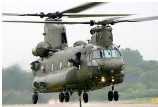
Ch47 Chinook helicopter with tandem rotors
